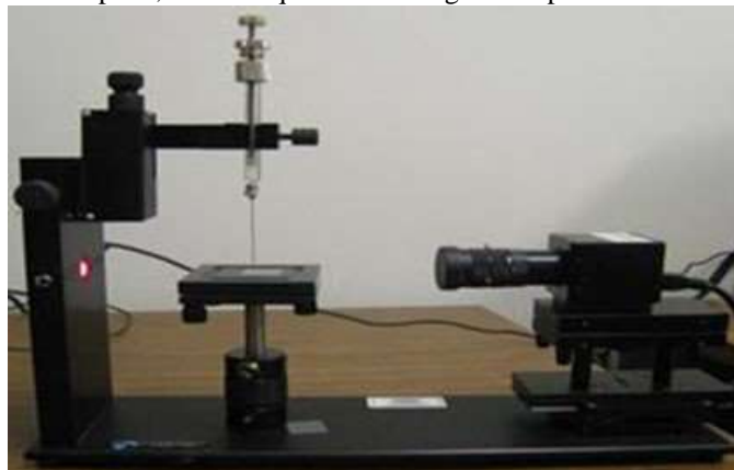
Figure 3: The photograph showing the optical contact angle goniometer used in the present study.
